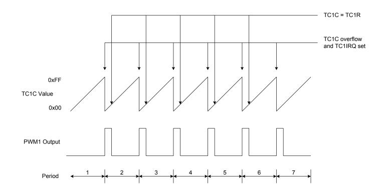
Above diagram is shown the waveform with fixed TC1R. In every TC1C overflow PWM output "High, when TC1C≧ TC1R PWM output "Low". If TC1R is changing in the program processing, the PWM waveform will became as following diagram.
