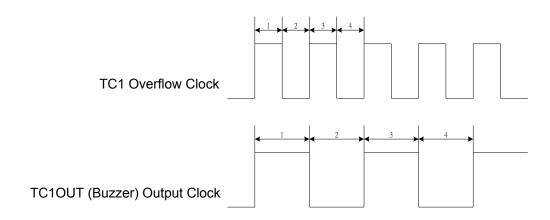
Example: Setup TC1OUT output from TC1 to TC1OUT (P5.4). The external high-speed clock is 4MHz. The TC1OUT frequency is 0.5KHz. Because the TC1OUT signal is divided by 2, set the TC1 clock to 1KHz. The TC1 clock source is from external oscillator clock. T0C rate is Fcpu/4. The TC1RATE2~TC1RATE1 = 110. TC1C = TC1R = 131.
