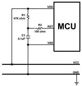
This is the basic reset circuit, and only includes R1 and C1. The RC circuit operation makes a slow rising signal into reset pin as power up. The reset signal is slower than VDD power up timing, and system occurs a power on signal from the timing difference.
