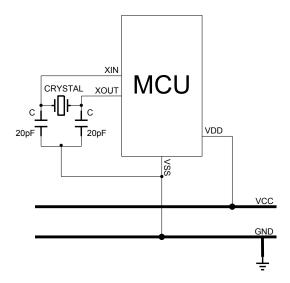
\* Note: Connect the Crystal and C as near as possible to the XIN/XOUT/VSS pins of micro-controller.
