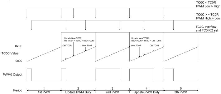
In period 2 and period 4, new Duty (TC0R) is set. TC0 is double buffer design. The PWM still keeps the same duty in period 2 and period 4, and the new duty is changed in next period. By the way, system can avoid the PWM not changing or H/L changing twice in the same cycle and will prevent the unexpected or error operation.
