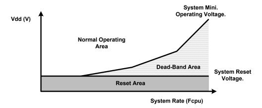
Normally the system operation voltage area is higher than the system reset voltage to VDD, and the reset voltage is decided by LVD detect level. The system minimum operating voltage rises when the system executing rate upper even higher than system reset voltage. The dead-band definition is the system minimum operating voltage above the system reset voltage.
