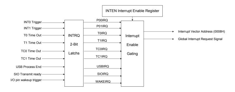
Note: The GIE bit must enable during all interrupt operation.
